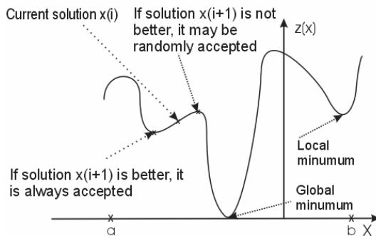
**Fig. 2** Principle of finding the global minimum of a quality index via the simulated annealing algorithm, where  $x$  represents vector of solution  $(k, q)$
