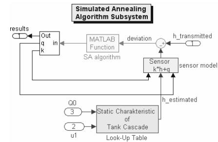
**Fig. 5** Simulated annealing algorithm subsystem
