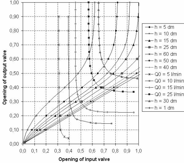
**Fig. 4** Steady-state characteristic of a two-water-tank cascade, where  $h$ ,  $Q_0$  corresponds to the estimated water level, respectively to the volume rate of flow
