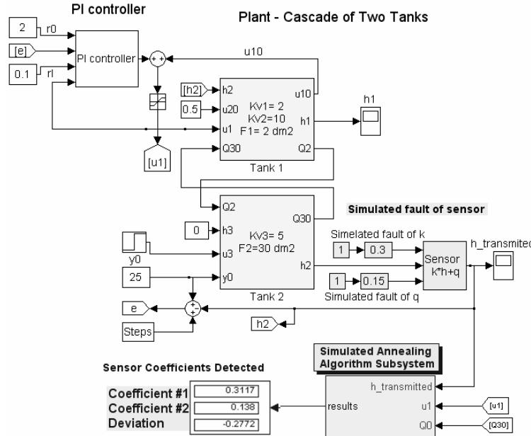
Fig. 3 Simulation scheme for auto-detection of sensor discredibility in Matlab/Simulink software
